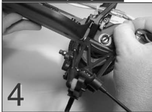
Locking The Diff Screw And Outdrive for Adjusting
