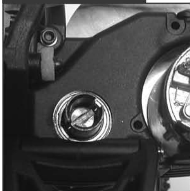
Line Up Slots In Diff Screw & Outdrive
